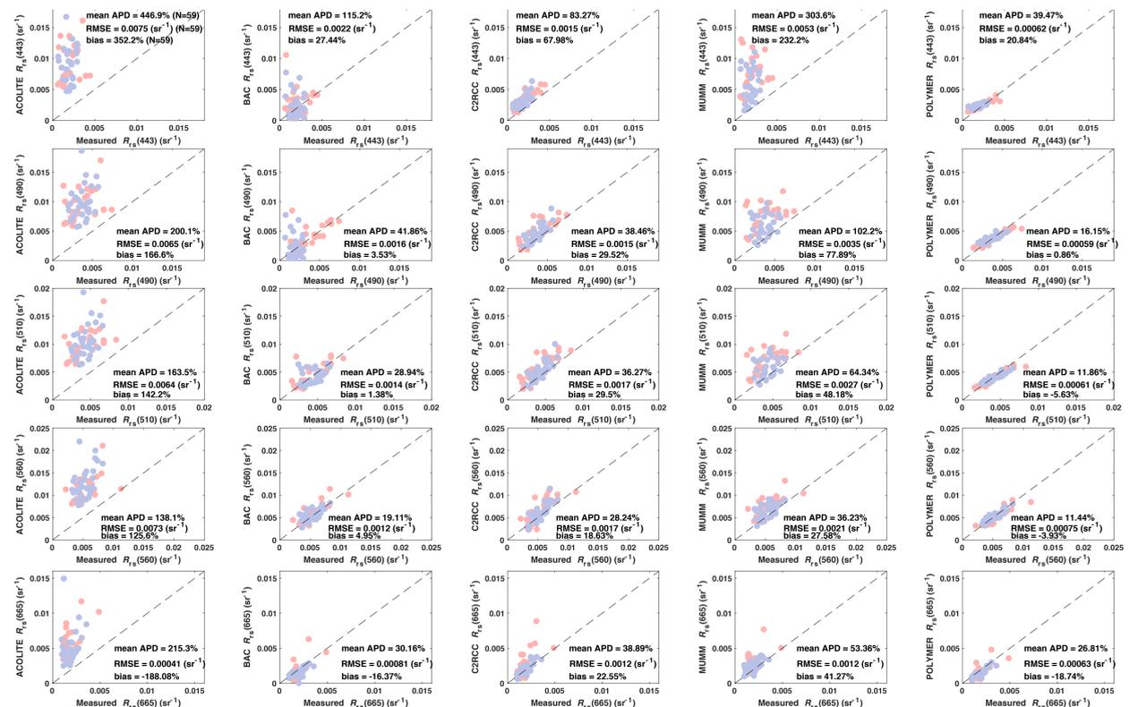
Fig. 3. Result of the five atmospheric correction approaches applied to the LIS region. Red symbols indicate time series Rrs data obtained from AERONET-LISCO fixed station (from 2016 to 2018) ; blue symbols indicate in situ Rrs data collected by our group (2018-now).
