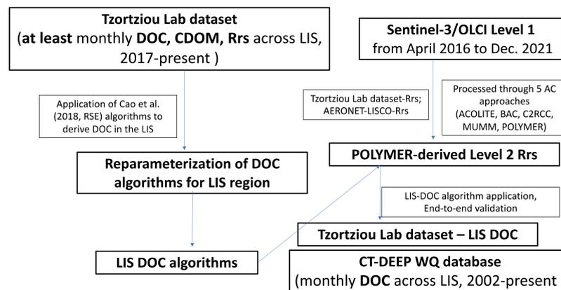
Fig. 2. Flow chart showing three steps: (1) Development of the LIS-DOC algorithm using our in-situ measurements collected in 2017-2021; (2) Processing of OLCI L1 data using different atmospheric approaches; and (3) end-to-end validation of LIS-DOC algorithms using CT-DEEP measurements of DOC concentrations and our in-situ measurements of both DOC concentrations and CDOM optical properties.
